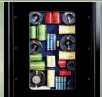
The top crossover equipment is visible from the rear through a Plexiglas window.
