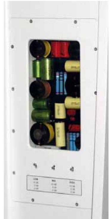
Fine separation: The imposingly equipped mid to high portion of the frequency separating filter can be seen at work behind the plexiglass. The toggle switches underneath adjust the level.
