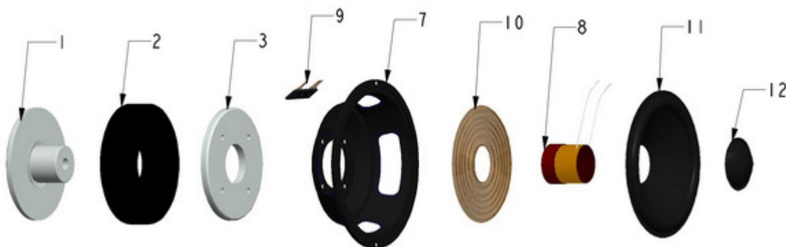
TAGA paper cone driver with oversized magnet ( $\Phi 100$  F models ;  $\Phi 80$  CS model), cloth dust cap and heavy duty combo T-yoke, voice coil and coil former with high purity wiring, is responsible for high power handling as well as deep, precise and detailed bass (and detailed, rich and spacious midrange frequencies in mid-woofers models).
