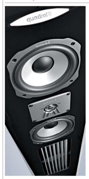
which claims to enhance the bass frequency response. It makes use of a bass reflex port along with membrane vibrations of the midbass drivers. It is called a pressure chamber as it is practically a section within the cabinet that houses two out of the four midbass drivers used in the speakers.
