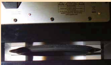
The Quadral subwoofer chassis is fitted between the bottom of the case and the base plate.
