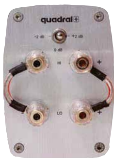
Superb: The bi-wiring connection terminals fitted on the Vulkan VIII R enable large speaker cables to be attached. The high tone level can be switched up or down by two decibels.
